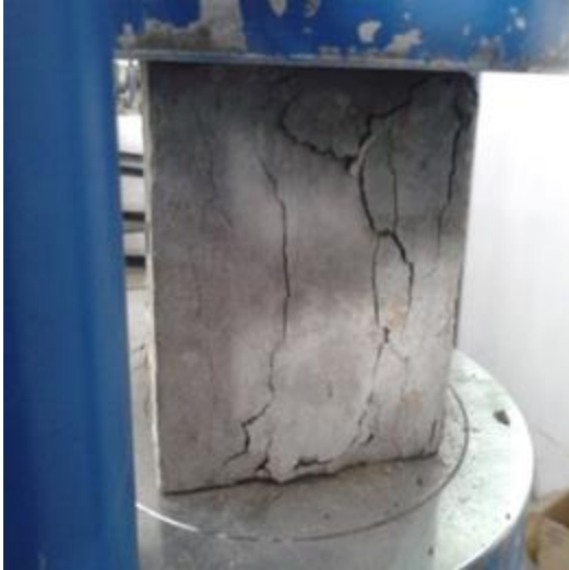
Fig. 5.2 Cube after testing
