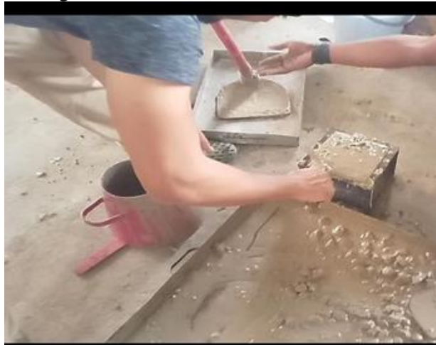
Fig.8 Casting of specimen
