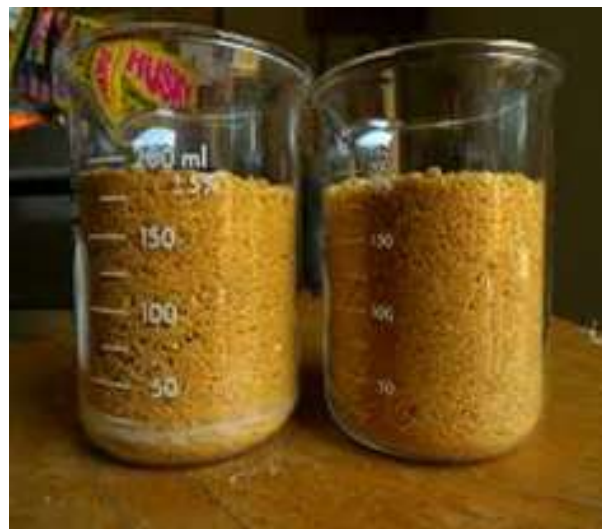
Figure 13 Bulking of sand
