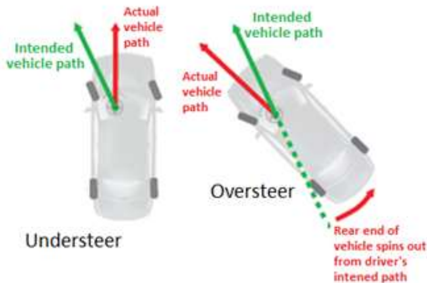
Figure 1: Understeer and oversteer conditions in vehicle dynamics. Adapted from Miroslav Demic, A Car in Understeer and Oversteer Conditions (ResearchGate, 2017). Retrieved from ResearchGate
