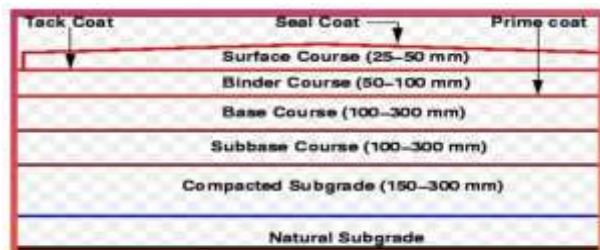
Figure 1.1. Cross-sectional view of flexible pavement.
