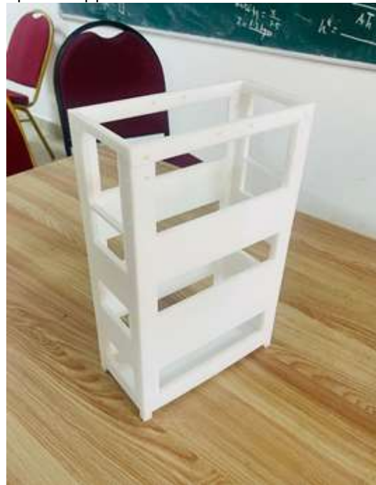
Fig 3: OUTER CASE of Nanosatellite made with (PETG)
