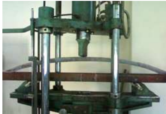
Fig. 6 Load applying on GFRP Leaf spring
