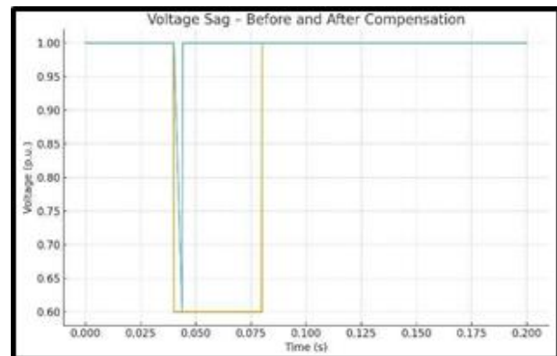
Figure shows 7a Voltage Sag – Before and After Compensation
