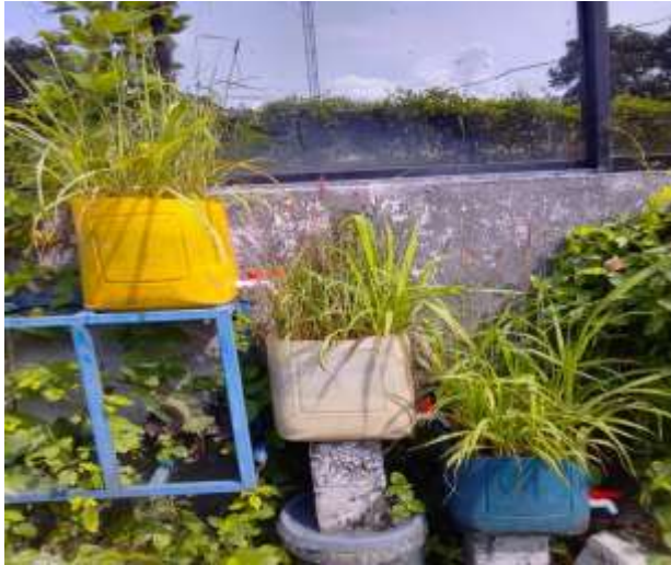
Figure 1: A 3-reactor constructed wetland in series for produced water treatment
