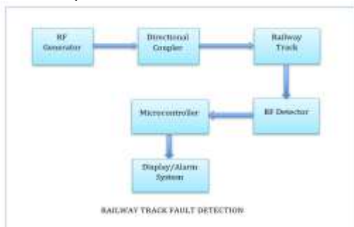
Fig. 1. Block diagram of Railway track fault detection system
