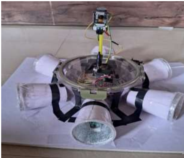
Fig. 10(a). Fully assembled AniDet prototype; six tubular shrouds at 60° spacing house the radar modules.
