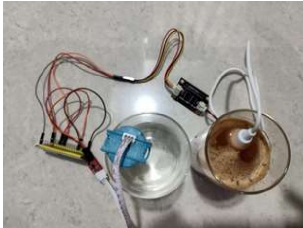
Fig. 1. SWPAS Hardware Prototype – Arduino/ESP32 microcontroller board (left), TDS sensor in clean water (centre), Turbidity sensor in contaminated water (right).
