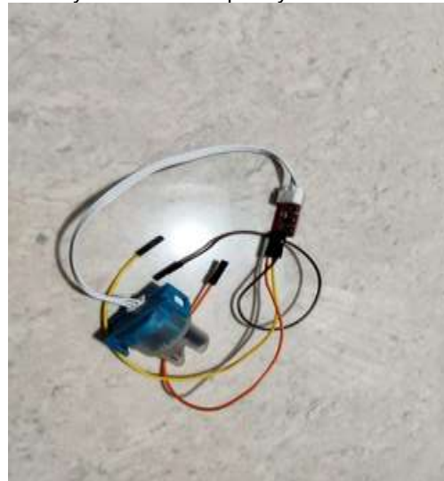
Fig. 3. Turbidity Sensor (blue probe) with signal board and wiring connections to ESP32.
