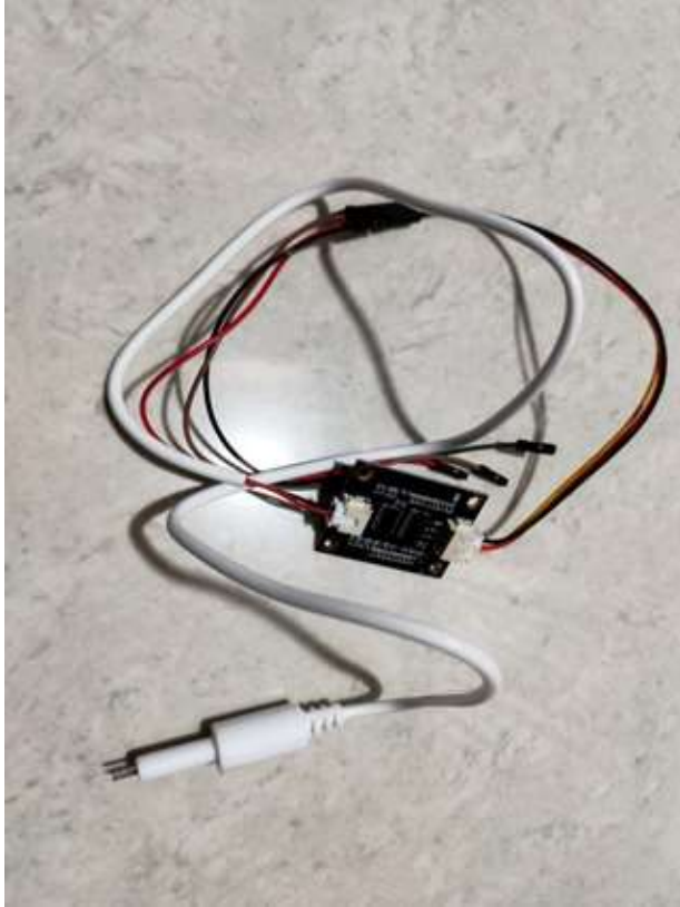
Fig. 2. TDS Sensor Module with signal board and jumper wire connections to ESP32.
