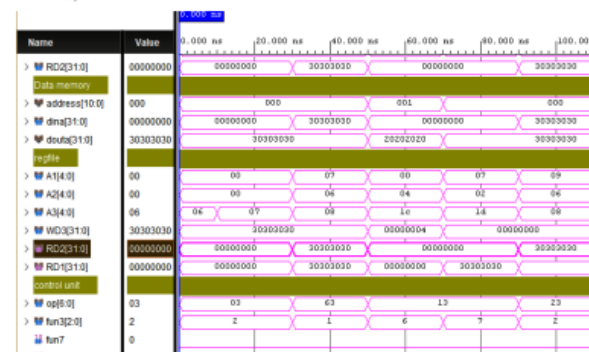
Fig. 4. Output of single cycle processor(Data memory and Register file)
