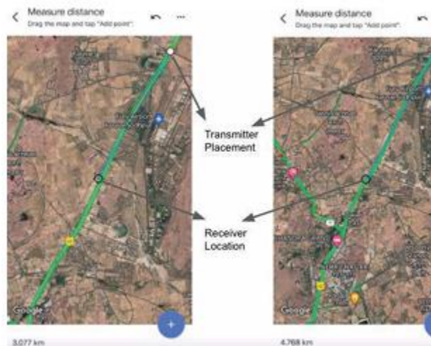
Fig. 6: Picture of the maps showing the achieved communication range for 100% data reception and 20% data reception.
