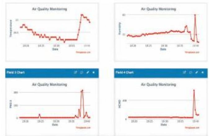
Fig. 2: Results of the implemented air quality monitoring system as seen on the ThingSpeak platform data.
