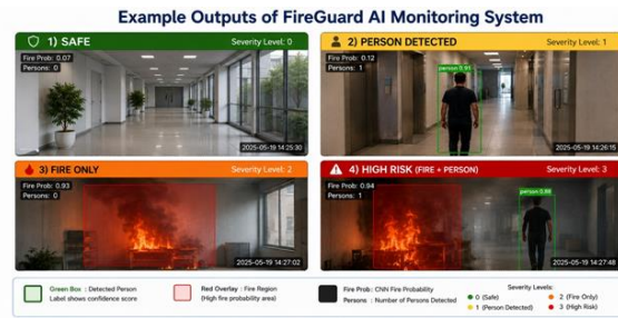
Figure 7. Example outputs generated by the FireGuard AI monitoring system under different threat conditions.
