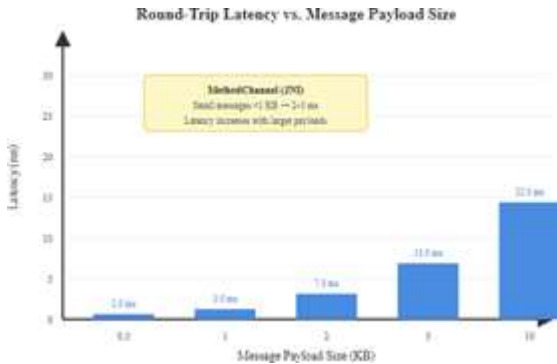
Fig. 11. Bar chart showing measured round-trip latency for different message payload sizes (0.5KB, 1KB, 2KB, 5KB, 10KB)
