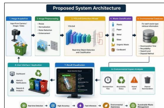
Figure 1. Proposed System Architecture of the YOLOv8-Based Waste Classification Framework.
