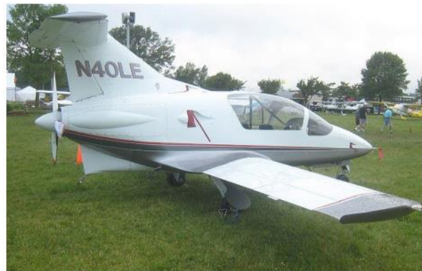
Figure 4. Rear/tail-mounted pusher propeller configuration on the Prescott Pusher (USA).
