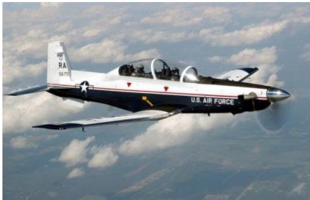
Figure 2. Nose-mounted propeller configuration on the Beechcraft T-6 Texan II trainer aircraft (USA).
