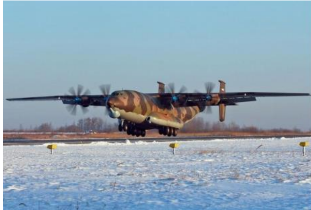
Figure 5. Four-propeller configuration on the An-22 heavy transport aircraft (Russia).
