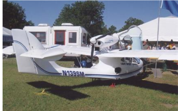
Figure 3. Fuselage-mounted propeller configuration on the SeaMax M-22 (USA).
