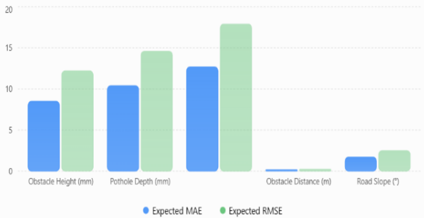
Fig. 4. Expected MAE and RMSE of the proposed road geometry estimation module for obstacle height, pothole depth, obstacle width, obstacle distance, and road slope.
