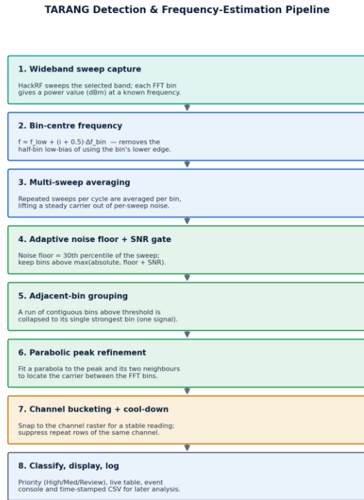
Fig. 6. The TARANG detection and frequency-estimation pipeline, from wideband sweep capture through to classification, display, and logging.
