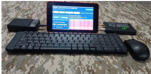
Fig. 5. Field configuration of TARANG: a tablet-class computer running the application, a portable battery, and a HackRF Pro SDR. The complete kit is carried and operated by a single person.
