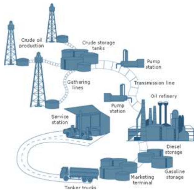
Figure 1. Diagram of the Crude Oil Refinery Supply Chain
