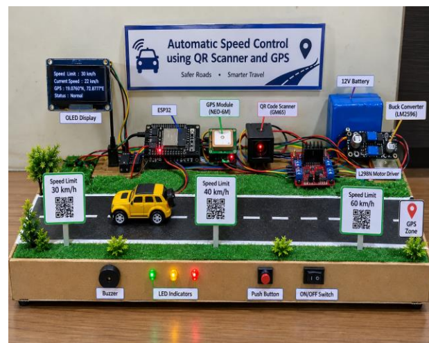
Figure 1: Automatic Speed Control System
