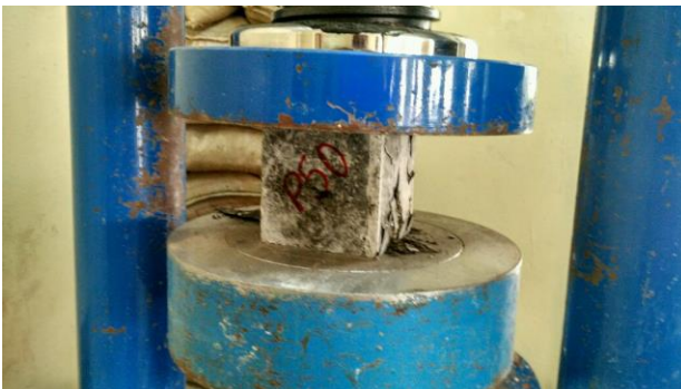
Fig. 3. Compression testing of cube specimen
