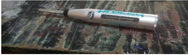
Fig. 9. Rebound hammer used for non-destructive testing
