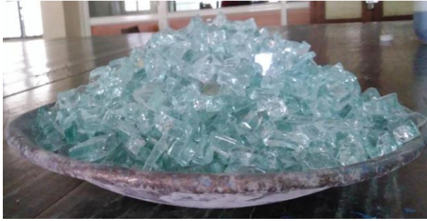
Fig. 1. Waste glass used as coarse aggregate
