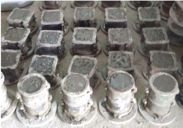
Fig. 2. Cast concrete specimens
