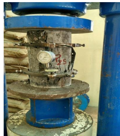
Fig. 8. Elastic modulus / cylinder test setup
