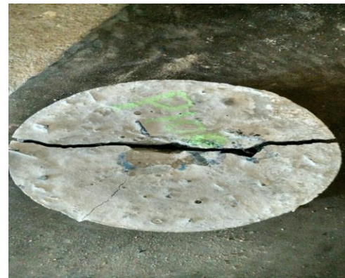
Fig. 6. Impact-test disc after cracking
