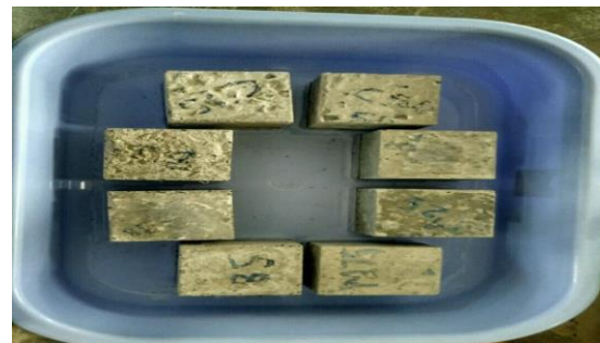
Fig. 7. Sorptivity specimens during water exposure
