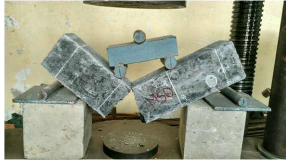
Fig. 5. Flexural test setup
