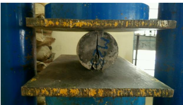
Fig. 4. Splitting tensile test setup
