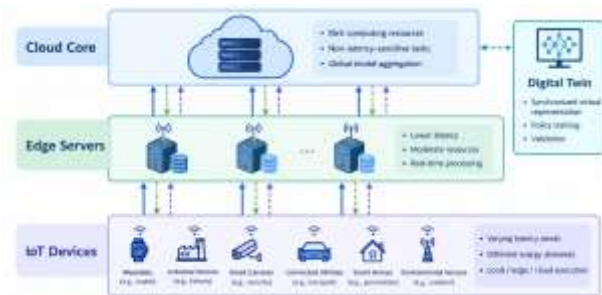
Figure 1: Proposed AI-driven adaptive resource allocation architecture
