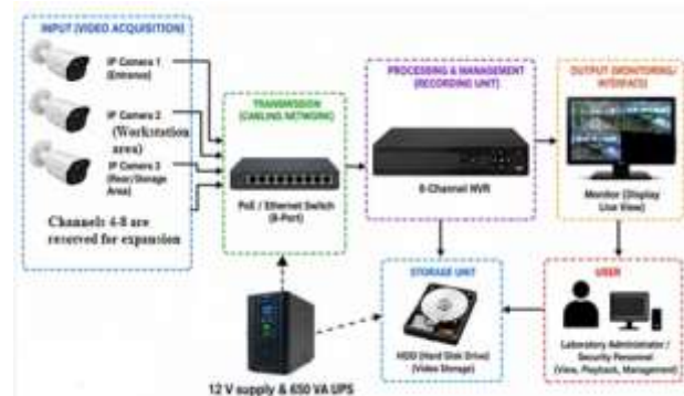
Figure 1. Architecture of the ELSMS. Three IP cameras (1–3) connect through a Gigabit Ethernet/PoE-capable switch to an 8-channel DVR with a 1 TB surveillance drive; channels 4–8 are reserved for expansion. The power path (dashed lines) runs through a regulated 12 V supply and a 650 VA UPS
