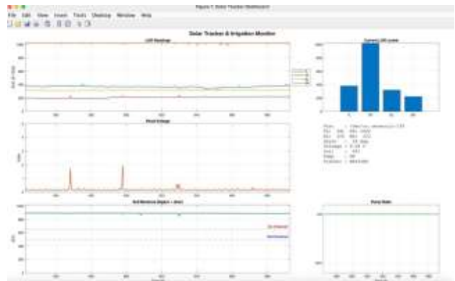
Figure 6: MATLAB “Solar Tracker & Irrigation Monitor” dashboard (screenshot of captured live data, about 545–693 s). Top row: LDR trends and current LDR bar graph; middle row: panel voltage and status text; bottom row: soil moisture with dry (650) and wet (500) thresholds, and pump state. Status text: TL 381, TR 1022, BL 320, BR 223, servo 26°, voltage 0.20 V, soil 891, pump ON, tracker WAITING.
