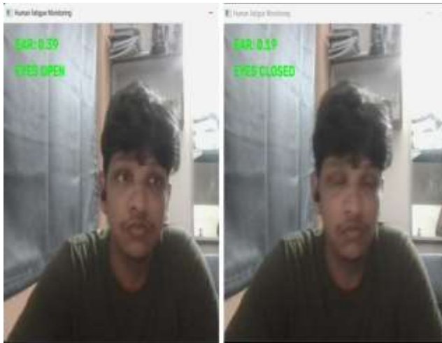
Fig. 2. Example open-eye frame (EAR = 0.39) and closed-eye frame (EAR = 0.19) from the implemented vision prototype.
