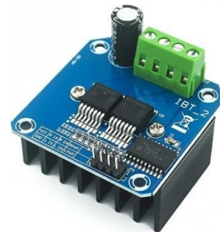
Figure 4: Motor Driver DC Gear Motors
