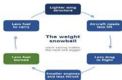
Figure 15.1: The weight snowball. A saving in structural weight grows as it passes through the aircraft design.
