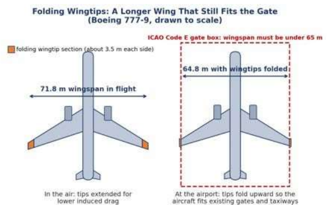
Figure 6.2: The Boeing 777-9 with its wingtips extended for flight (left) and folded at the gate (right), drawn to scale. The folded span fits within the 65-metre limit of an ICAO Code E gate.
