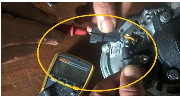
Fig 8 Blocking diode Open circuit noticed inside the plug molding.
