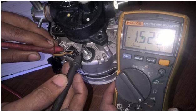
Fig 7 In multimeter checking at WL & W point in the rectifier assembly – Alternator found intact
