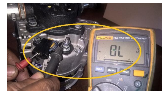
Fig 6 Open circuit noticed between WL Positive terminal and W terminal to Ground in the alternator.
