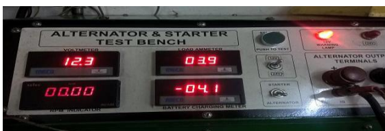
Fig 10 Battery indicator glow on in the LIS test rig.
