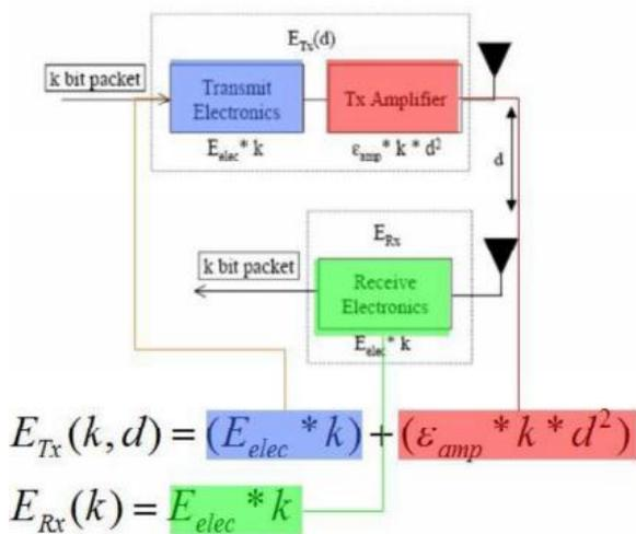
Fig. 1 Radio Model of D-LEACH.
