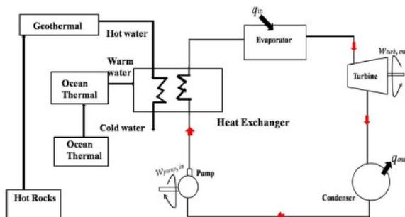
**Figure 3:** Geothermal electric generation system.
