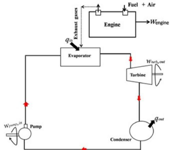
Figure 1: ORC in waste heat recovery.
