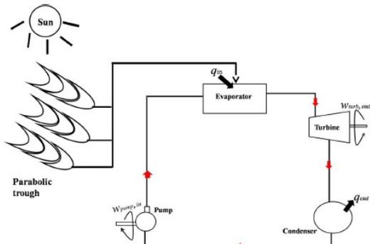
**Figure 2:** Solar thermal power plant.
