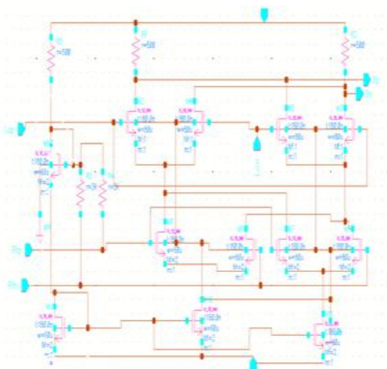
Figure 16: 16.Schematic of Double Trans conductance stage Mixer.
