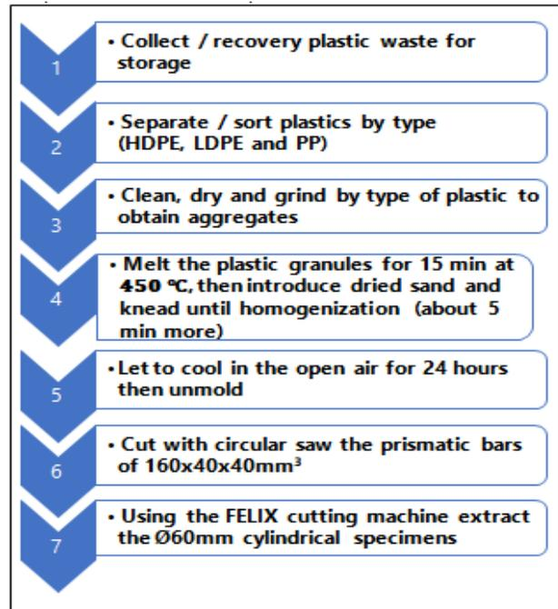
Figure 5: Methodology for manufacturing test specimens.
