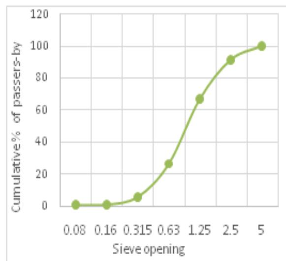
**Figure 2:** Granulometry curve of the sand used.
