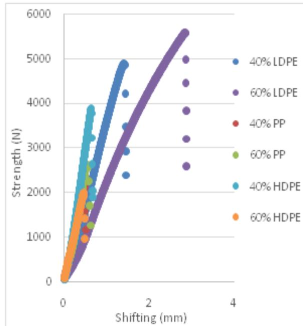
**Figure 9:** Three-point bending test curves.
