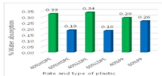
**Fig.8** Water absorption of specimens depending on the type and rate of plastics.
