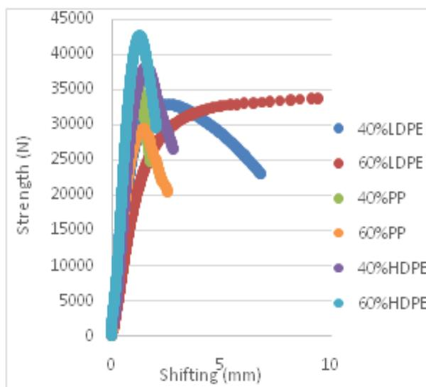
**Figure 11:** Compression test curves.
