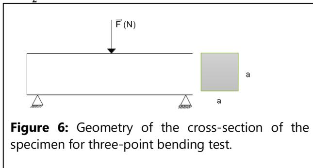
**Figure 6:** Geometry of the cross-section of the specimen for three-point bending test.
