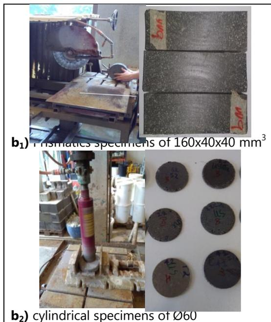
Figure 4: Presentation of FELIX test specimens, circular saw and cutting machine.
