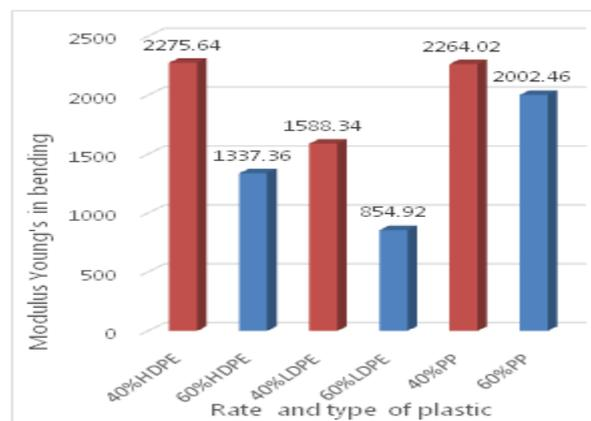
**Figure 10:** Variation of the Young's modulus according to the rate and type of plastic.
