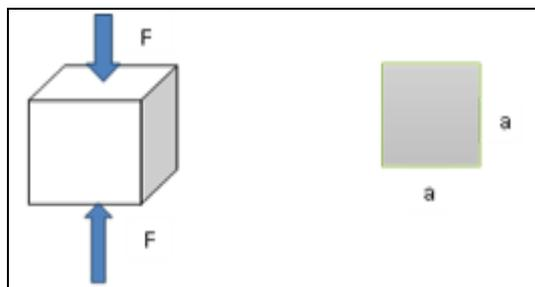
**Figure 7:** Experimental arrangement for compression test.
