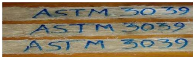
Figure 7: Test specimens were prepared using the band saw in Africa Bamboo Lab, Addis Ababa, Ethiopia.
