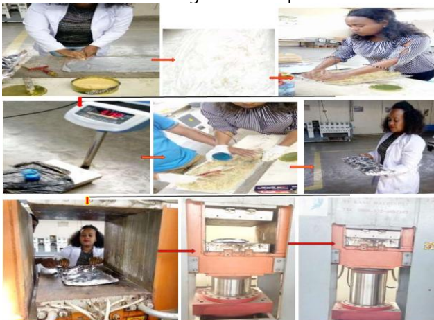
Figure 5: Palm fiber- epoxy resin mixture in the mold surface at Africa Bamboo Lab, Addis Ababa, Ethiopia. Prepared samples from palm leaves 15/85 composition of sample (15% fiber to 85% epoxy).
