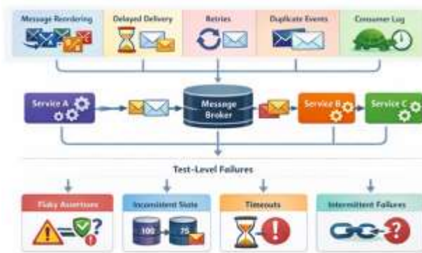
Figure 1: Failure Modes and Sources of Non-Determinism in Event-Driven System-Level Tests
