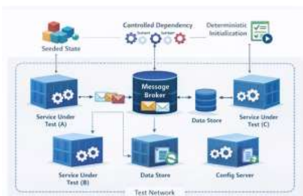
Figure 2: Reproducible Containerized Test Topology for Event-Driven Microservices
