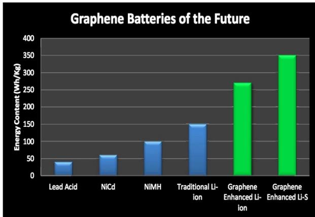
The lead-acid batteries was introduced in 1850's with energy density of 30-40wh/kg and charge discharge efficiency of 50-95%.
