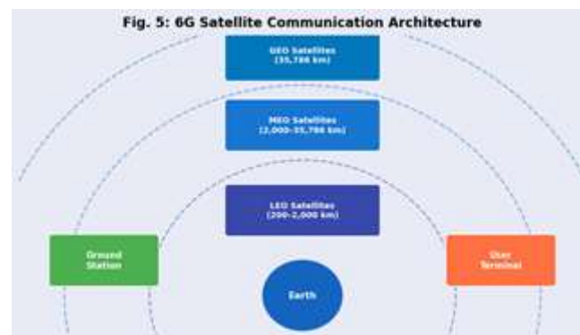
Fig. 5: 6G Satellite Communication Architecture integrating LEO, MEO, and GEO Orbits
