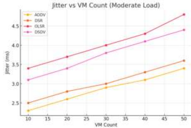
Figure 6. Jitter vs VM Count (Moderate Load). Reactive protocols (AODV, DSR) maintain lower jitter levels, while proactive protocols (OLSR, DSDV) show higher variability under virtualization overhead.
